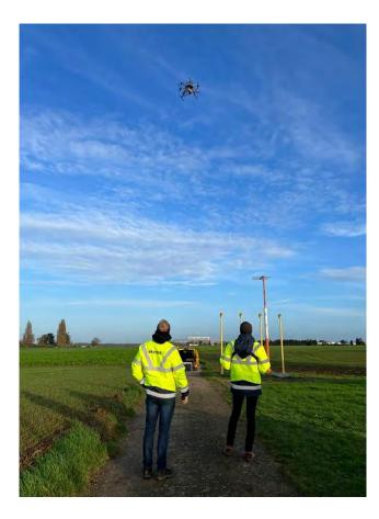
of advantages. As drones are more flexible and lighter, their use makes it possible to reduce the number of inspection flights, thereby cutting costs and preserving airport capacity. skeyes acquired a specialised drone in 2021, finalised the procedures for its use in 2022 and started operational inspections in 2023.
